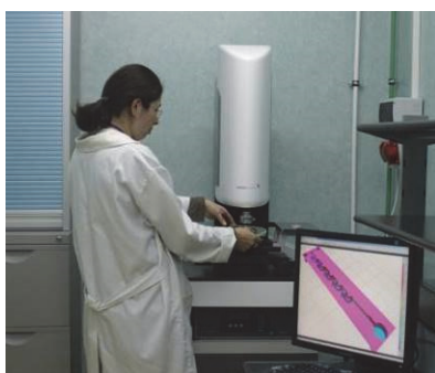
White Light Interferometer - Photomap 3D (FOGAL nanotech, France)
