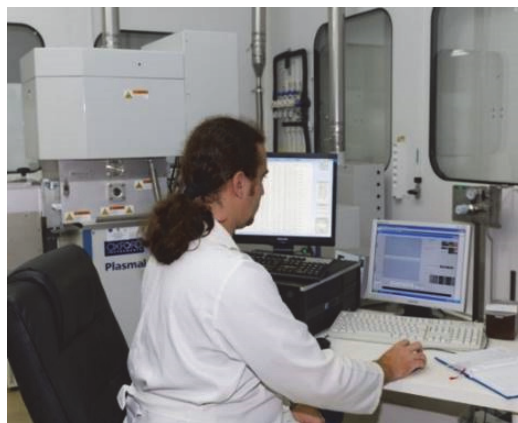
DRIE - PlasmaLab System 100 (Oxford Instruments, UK)
