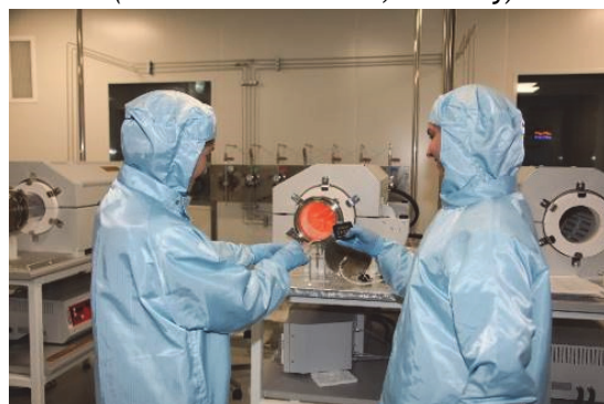
RIE Plasma Etcher - Etchlab 200 (SENTECH Instruments, Germany)
